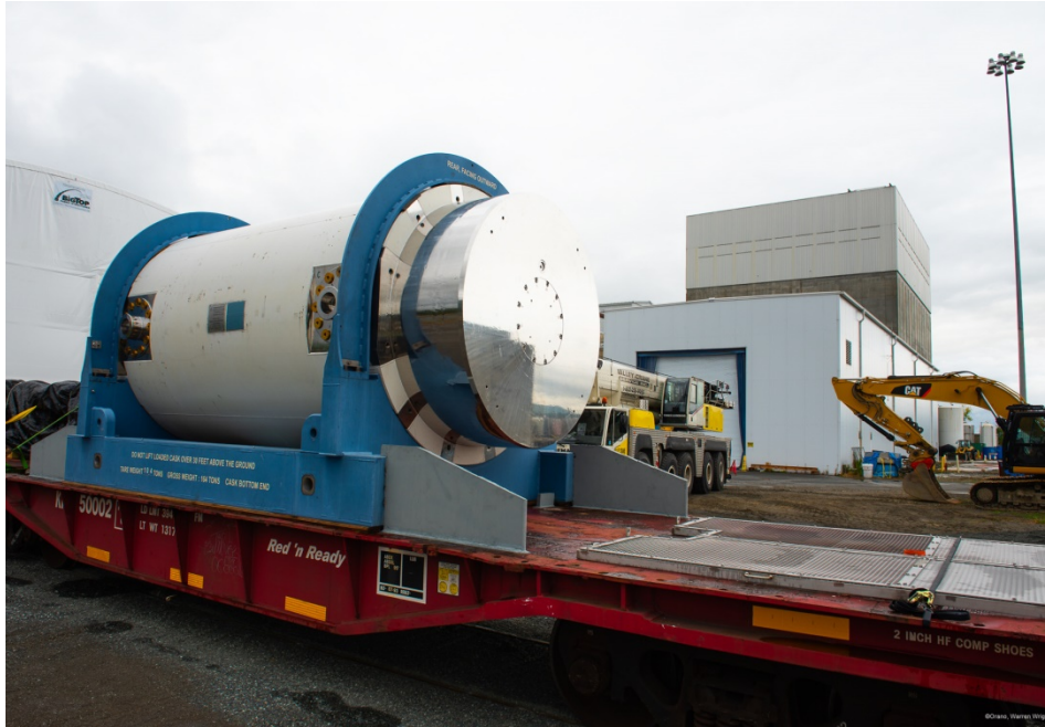
Onsite at the Vermont Yankee accelerated decommissioning project, Orano's MP197HB shielded transport cask is one several methods for waste packaging and transport, according to the content's characteristics. Image: © Orano, Warren Wright.
